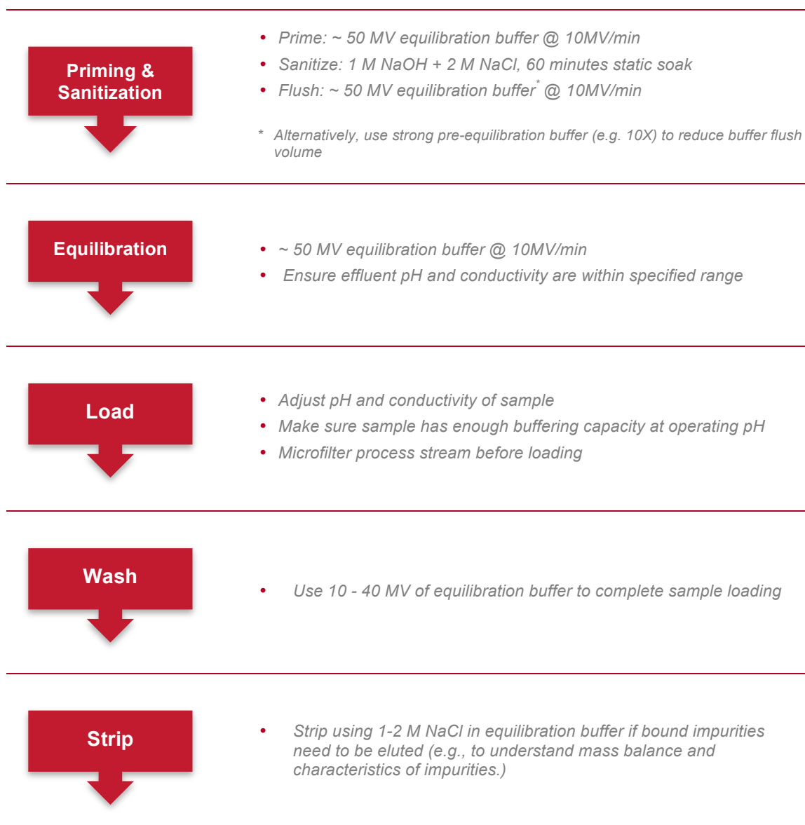
Figure 1: Steps in NatriFlo HD-Q chromatography
